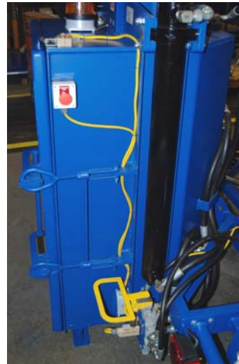
FIG. 6: Open the door to the drum enclosure to separate the 2 sides of the door switch. Cover the contact surfaces of both sides with electrical tape, close and latch the door, and then try to lower the crusher ram.
