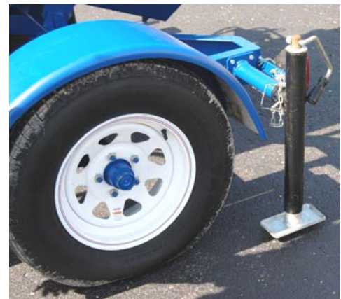
FIG 8B: Fasten the jacks to the jack mounts with the retaining pins.
