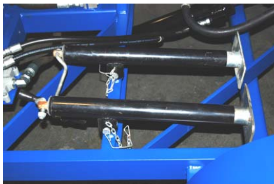
FIG 8A: Disconnect stabilizing jacks from storage couplings; remove the retaining pins; then pull the jacks upwardly to uncouple them from the trailer.
